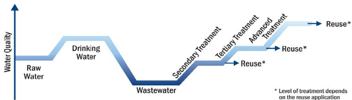
Figure 1. Treatment technologies are available to achieve any desired level of water quality (Guideline for Water Reuse, EPA 2012)
