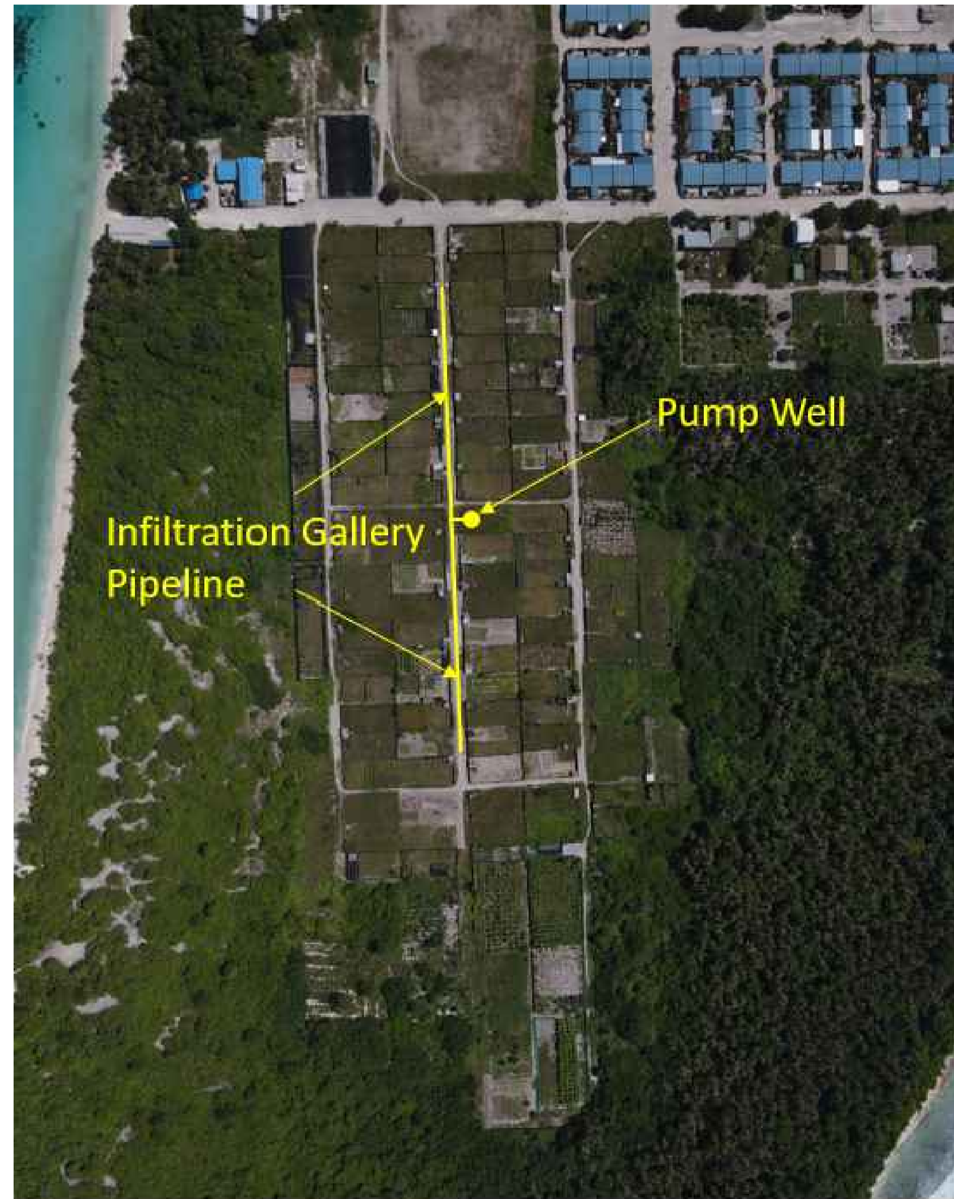
INFILTRATION GALLERY GENERAL ARRANGEMENT
