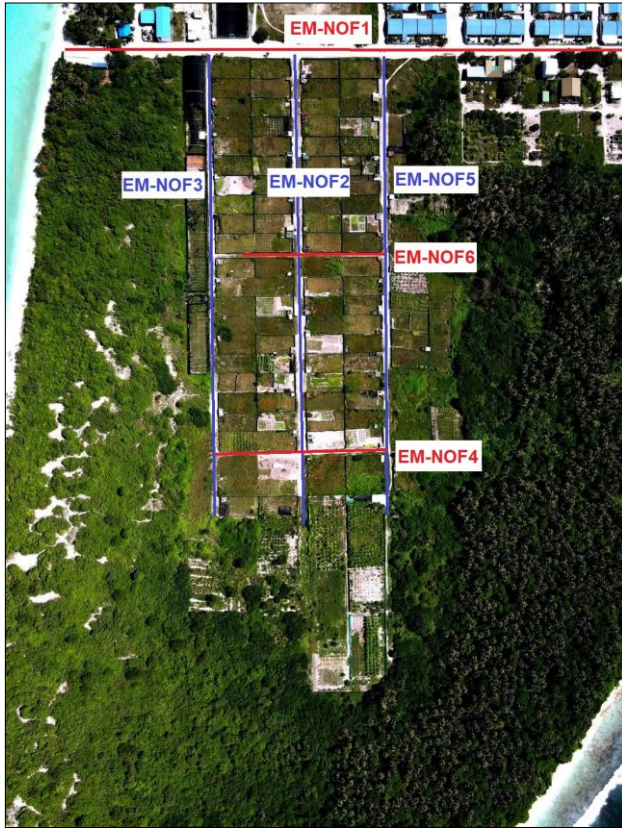
Figure 6 Image from drone showing agricultural plots and locations of six EM surveys
