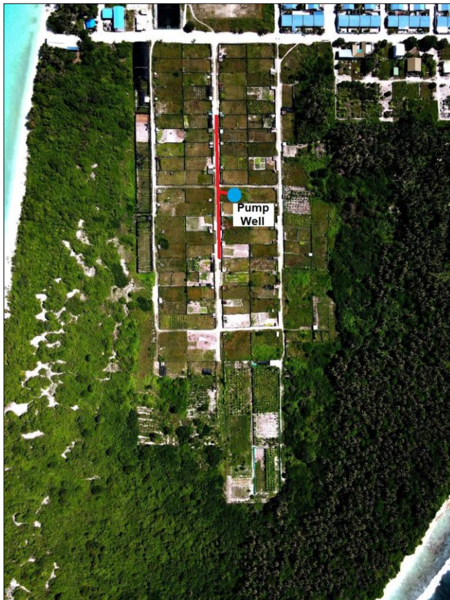
Figure 20 Image from drone showing proposed location of gallery (shown in red with blue offset pump well)
