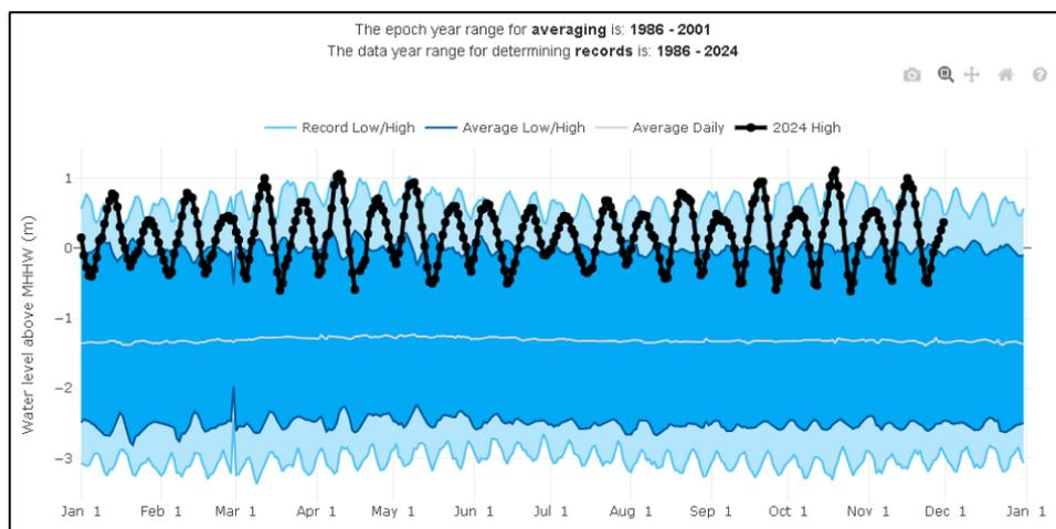
Figure 12: Monthly Means of the observed tidal heights in 2024 for Kilindini area of Mombasa
