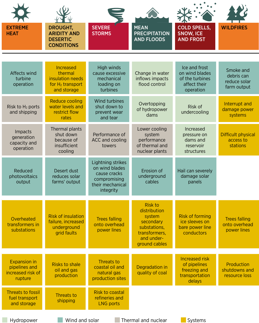
FIGURE 3.9 Exposure of electricity generation assets, network and supply chains to climate-related risks
