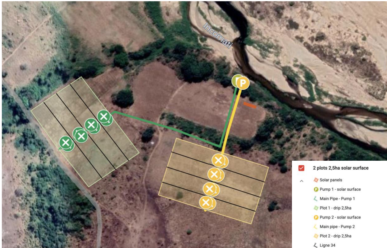
Figure 1. The geometry of the proposed irrigation system in the Pangalata association.
