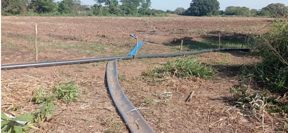
Figure 5: Lay flat hose used to pump water into the field from pump.
